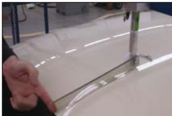
ALIGN POLYCARBONATE GAUGE WITH TOP EDGE OF WINDSHIELD TO LOCATE THE CALIBRATED GAUGE AT EXACTLY 10 INCHES BACK FROM THE WINDSHIELD.
