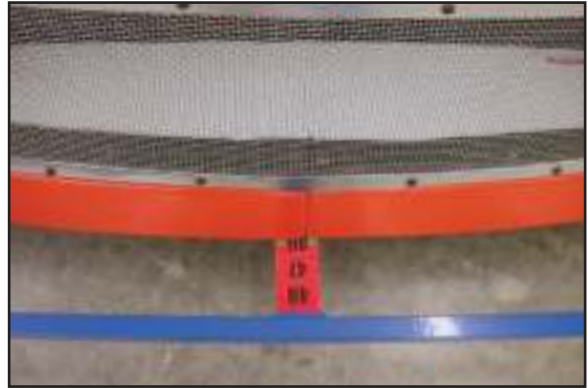
FRONT OVERHANG IS MEASURED BY VIEWING THE GAUGE AT THE BASE OF THE NOSE.
