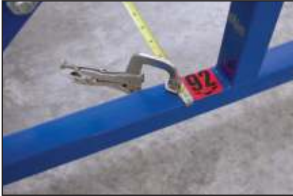
CLAMP TAPE MEASURE TO OUTSIDE OF ONE SIDE OF DEVICE.
